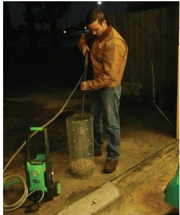
Figure 9. Removal of peanut exocarp using water with an electric pressure washer.
