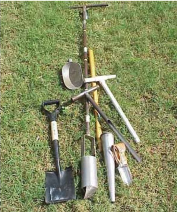
Figure 6. The collection of soil samples for nematode analysis can be acquired from the field using cylindrical sampling tubes, a trowel, a bucket auger, or a shovel.
