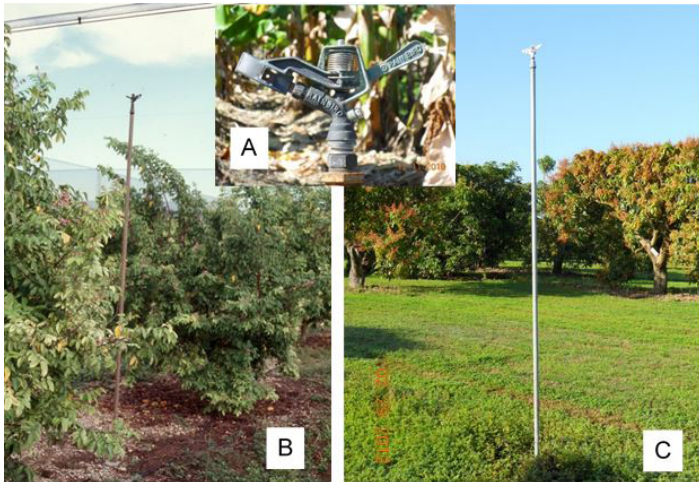
Figure 1. High-volume overhead irrigation pipe (metal pipe, 10 to 15 ft high) with brass high-impact sprinkler head (A) in a carambola grove (B) and a mango grove (C).
