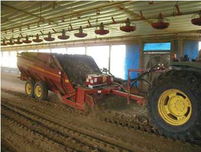
Figure 2. Machine used to scrape a layer of litter (manure and bedding) in the poultry house. Credits: J. Jones
