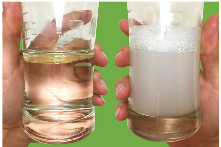
Figure 4. The left glass contains only oil and water, which rapidly separate after being shaken together. The same solution at right has been stirred and emulsified by a drop of detergent.
