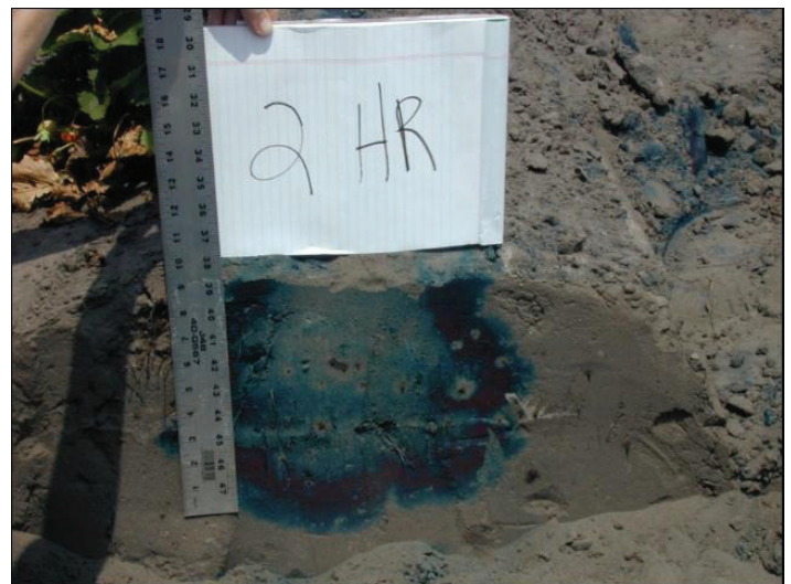
Figure 2. Cross section of beds after 2 hours of irrigation. Credits: J. R. Duval (2002)
