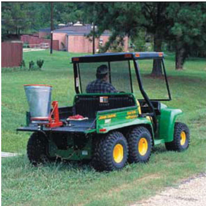
Figure 11. Man applying fire ant treatment with spreader attached to the back of a Gator utility vehicle.
