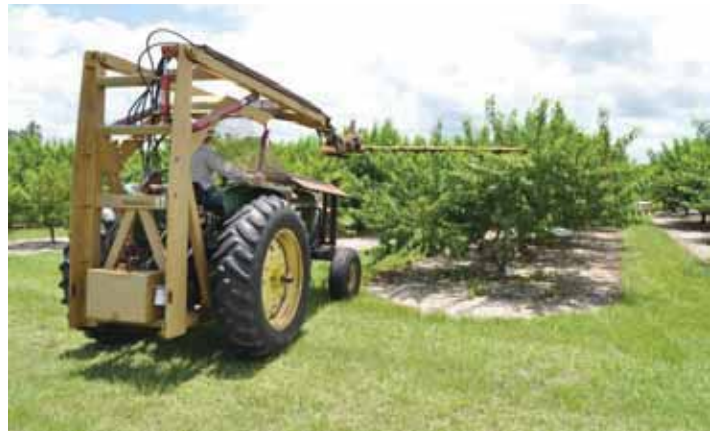
Figure 9. Cutting back the tree at a manageable height (6–8ft) using a disc pruning. Credits: D. Huff
